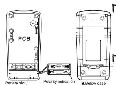
1. Remove the screws on the back of case and open the case.
