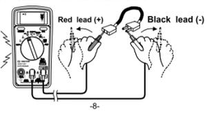
**Current Measurement ( $\mu\text{A}$  /  $\text{mA}$  /  $\text{A}$ )**
